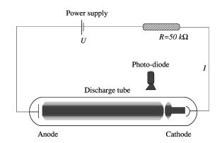
FIG. 1. Experimental setup. The light fluctuations are recorded near the cathode with a sampling rate of 500 kHz.
