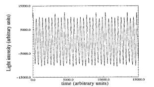
FIG. 2. Time series of the light intensity recorded near the cathode by using a photodiode (I=30.4 mA).
