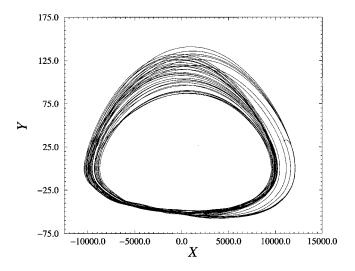
FIG. 3. Plane projection of the reconstructed phase space spanned by derivative coordinates (I = 30.4 mA).
