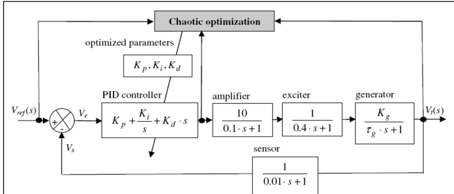
Fig. 2. Block diagram representation of an AVR system using a PID controller with chaotic tuning.
