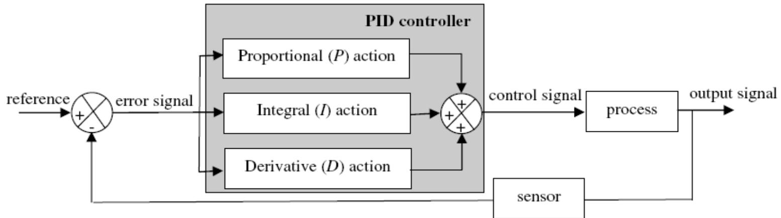
Fig. 1. Block diagram representation of a PID controller in a closed loop system.
