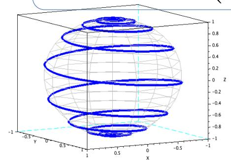
Motion on the Bloch Sphere ( $|M(t)| = \text{constant}$ )
