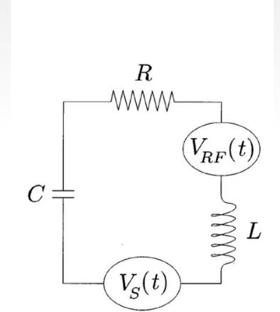
$$L \frac{d^2}{dt^2} i(t) + R \frac{d}{dt} i(t) + \frac{1}{C} i(t) dt = \frac{d}{dt} V_S(t)$$
